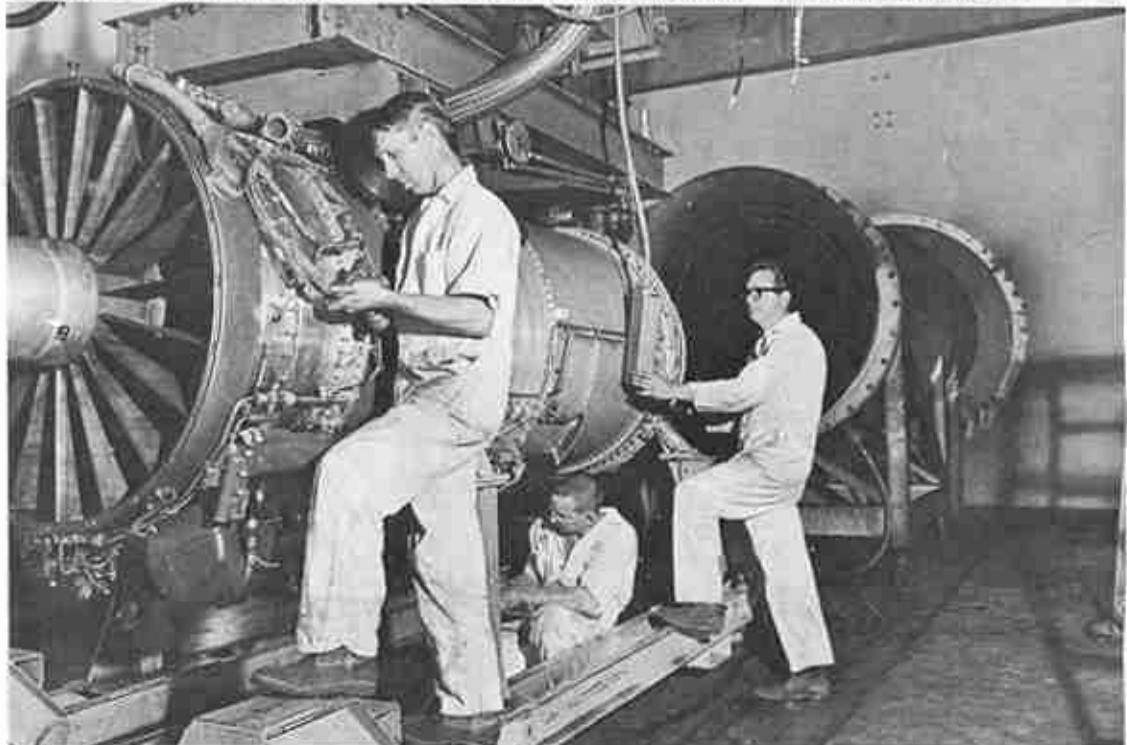
727 FAN JET engine is set up in a sound-proof cell by Ronnie Walters, left, Cookie Bennett, and Steve Hall, right. Hundreds of wires are connected to the engine during its test to insure proper functioning of all parts.
