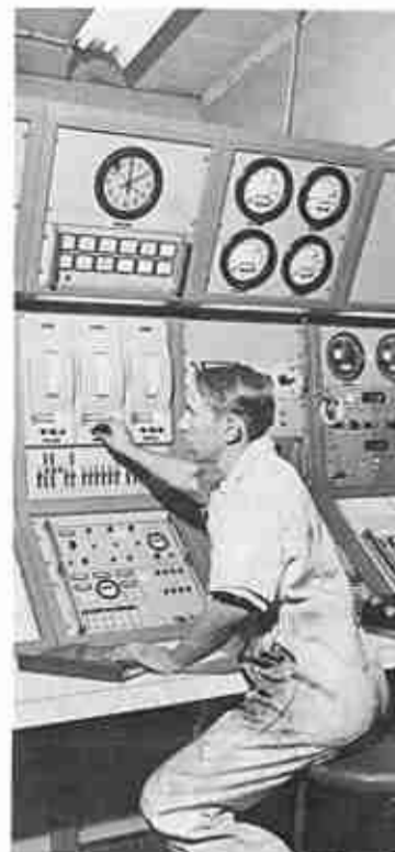
TEST CELL operator Ronnie Walters checks for 14,000 lbs of thrust on test panel which is outside cell block where all PSA engines are run for three hours before being replaced on aircraft.
